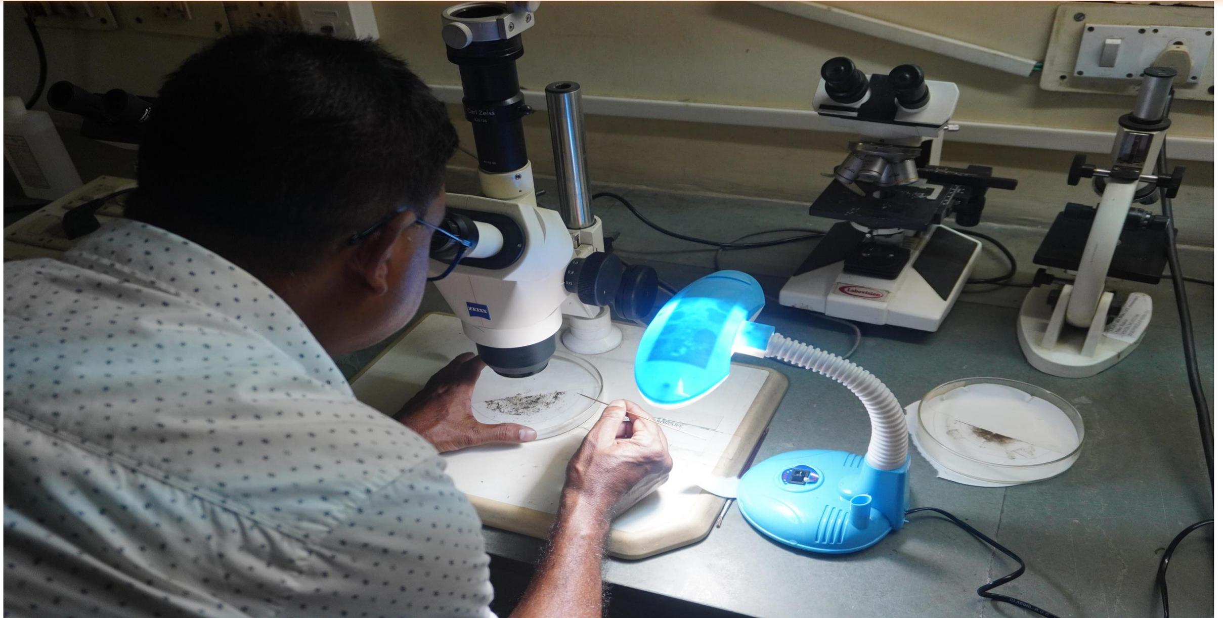
Demonstration on picking of AMF spores under microscope using a needle
